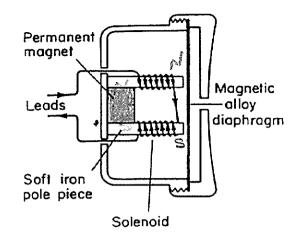
the sound waves. A similar electric current is caused to pass through the solenoids in the earpiece. This alters the strength of the magnetic flux in the U-shaped magnet and produces a corresponding variation in the pull of the diaphragm. The latter therefore vibrates and reproduces a copy of the sound waves which entered the microphone.
